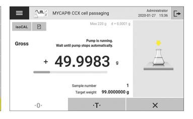
During sample processing the receiving flask is fixed on the balance weighing pan, the balance is tared and then the peristaltic pump transfers liquid from the donor flaks to the receiving flask. The volume to be transferred is automatically calculated by the software application and transformed into a target weight value using the media density.
