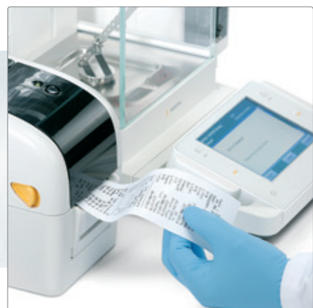
Step 5: Print the results in GLP or label form on self-adhesive paper
