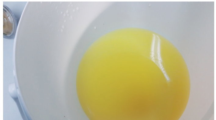
Fig. 3: Defined clay-suspension: 2.02 g clay/2 L, homogenized using a disperser, with a turbidity of 910 NTU on average.
