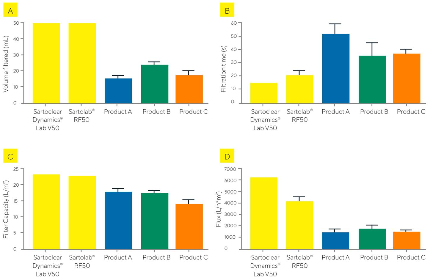
**Figure 2:** Filtration performance of Sartoclear Dynamics® Lab V50, Sartolab® RF50 and products A, B, and C. A: Volume filtered until filter clogging occurred (max. volume 50 mL); B: Filtration time (until filter clogging); C: Filter capacity given in L/m<sup>2</sup>; D: Flux given in L/m<sup>2</sup>h. Shown here are the mean values of trials performed in triplicate, as well as the respective standard deviations.
