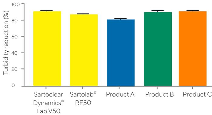
**Figure 3:** Turbidity reduction after clarification of the LV supernatant with Sartoclear Dynamics® Lab V50, Sartolab® RF50 and products A, B, and C. Shown are mean values of triplicates with standard deviations.
