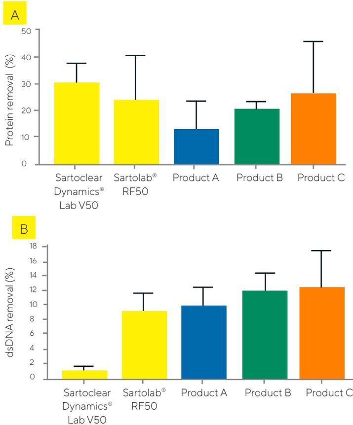
**Figure 4:** Protein (A) and dsDNA (B) removal after clarification of the LV supernatant using Sartoclear Dynamics® Lab V50, Sartolab® RF50, and products A, B, and C. Shown here are the mean values of the trials performed in triplicate, along with their respective standard deviations.
