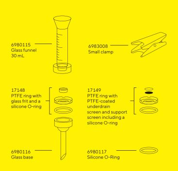
Note: PTFE rings in sets 17148 and 17149 have different dimensions and are not interchangeable.
