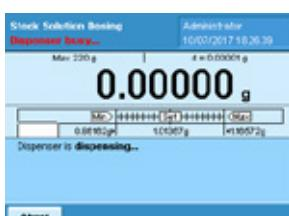
The solvent is automatically applied to the sample. During the dispensing step the message „Dispenser is dispensing“ is displayed to the user.
