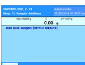
The test starts with the repeatability test. Press 'TARE' to begin the test.
