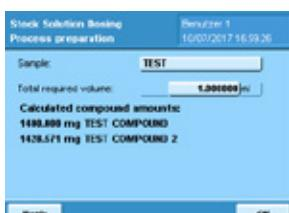
The total volume of the stock solution has to be entered. The final volume must not be higher than the capacity of the used vial.
