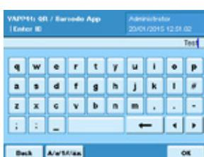
After the information is entered, press **OK** to output the code(s) on the YDP30 lab printer.
