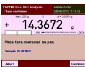
After pressing 'Initial weighing', you are prompted to place a tare container (e.g. a sample dish, or filter) on the weighing pan. After pressing 'Continue', the container is tared, the value is stored and the display is set to zero.
