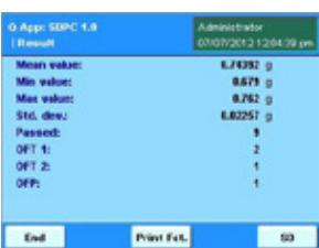
After reaching the "sample count" (number of products to be tested) or after pressing **Finish**, the final evaluation is displayed (OFP = out of plausibility).
