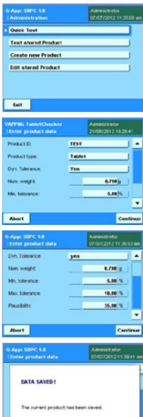
Entry level to create, edit or test products, additionally a non-stored product can be tested using the **Quick Test** option (e.g. to calibrate tablet pressing machines). This menu is only accessible for administrators!
