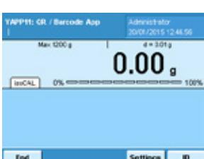
Press the **ID** button to select the input screen for entering a code.
