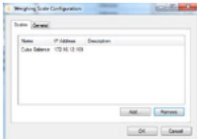
Enter the name and IP address of the balance. If necessary enter a descriptive text. To confirm the settings press „OK“
