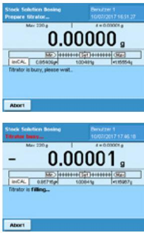
After the ventilation step is finished YAPP16 continues with the process and sends the required solvent volume to the dispenser.
