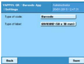
This application has been factory-set to "Barcode" as the type of code and to "continuous paper" as the type of label.
