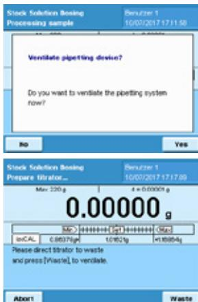
For the Hirschmann opus dispenser YAPP16 stores if a) the instrument has been properly ventilated to get rid of air bubbles and to fill the piston and if b) the residual solvent in the piston is sufficient to perform the next dispensing step. If that's not the case a message screen is shown to user with the question if the system should be ventilated.
