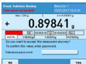
The user can accept or reject the result. If the administrator has activated the tolerance password approval, the user is forced to enter the password to accept out of tolerance values.
