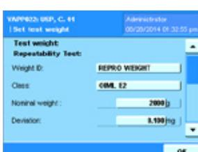
The Weight ID is an alphanumeric entry. The selection of the class is limited to OIML and ASTM weights. The input value of the weight is verified by the OIML and ASTM table.
