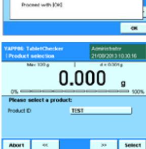
When starting the workflow with user permissions, or when entering via **Test stored Product**, the user is prompted to select (with <<, or >>) or enter (via keyboard or barcode scanner) the product ID needed to be tested.
