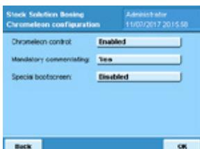
Chromeleon™ users must switch on the Chromeleon™ control of the Cubis dosing system. Chromeleon™ control enables the software to send and retrieve data to and from the balance.
