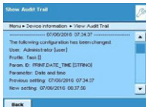
If the deviation between the NTP Server and balance time is larger than 2 seconds, the time will automatically be adjusted. After the adjustment, an Audit trail entry will follow.
