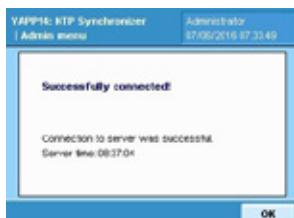
Press the 'Test' button in the configuration menu to check the connection to the NTP server. The time will be not changed at this test, it is just for checking the connection.
