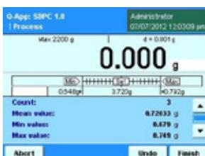
After the third measurement, ***Undo*** is displayed to undo the last product, in case of a handling mistake. The product will be taken out of the statistical analysis.
