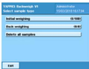
Main menu with the selection to weigh in samples, to weigh them back or to delete all samples from the internal memory (samples stay in the memory of the balance unless they are printed or sent to a FTP server). The numbers behind the menu points determine how many samples were already weighed in or back.
