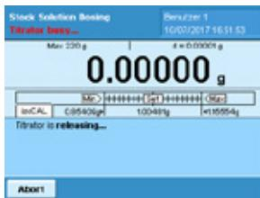
The solvent is automatically applied to the sample. During the dispensing step the message „Titrator is releasing“ is displayed to the user.
