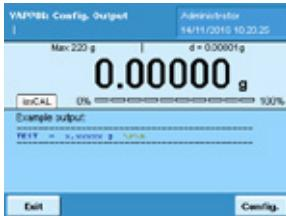
The start screen shows an example of the selected output format. Basically, the output format is divided into a name (header), a weight value and subsequent control characters.
