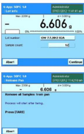
Entry of the **Lot ID** and the number of samples. When defining a certain number of samples, a Sartorius tablet feeder can be controlled to automatically feed the defined number of samples onto to weighing pan. If "0" is selected, the user defines the end of the process.
