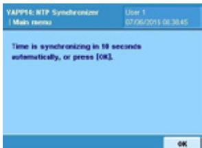
If a user without administrator rights is logged in, the Q-App can be started, but not ended manually. During the synchronization all hard keys except the on/ off button is blocked. This is for a fully automated use over a timer-controlled function, which is very convenient.
