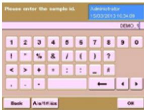
After pressing 'Initial weighing', you must enter the Sample ID (alphanumeric)
