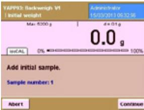
Afterwards, you are prompted to weigh in the first sample. The workflow automatically provides a sample number.
