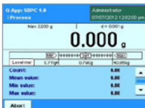
A checkweighing graph is displayed together with the statistical parameter, count, mean, min. and max values as well as the standard deviation (accessible by scrolling down).
