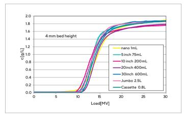
Break through curves of Sartobind devices with 4 mm and Pilot filter holder equipped with 13 Sartobind cassettes
