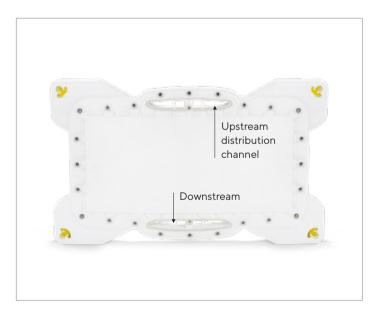
The side view of the cassette displays the upstream distribution channel where the feed enters between the two membrane stacks. The lower downstream channel collects the outlet of each cassette.
