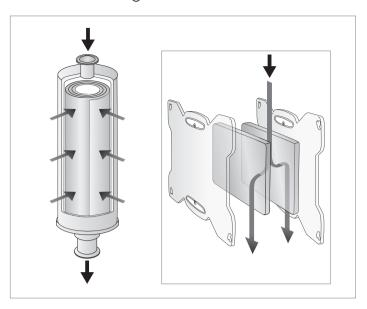
The cassette design is directly derived from the Sartobind capsules. Cutting and unrolling the membrane stacks results in two membrane stacks of 4 or 8 mm bed height. To achieve a small footprint, the stacks are unrolled. The feed enters between the membrane stack separated by a central spacer, flows through the membrane stacks and is collected at both sides of the outlet.
