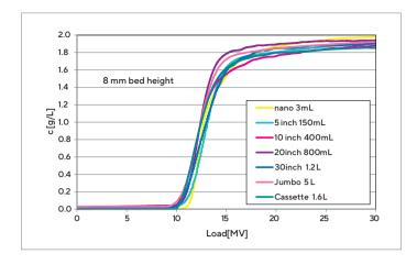
Sartobind devices 8 mm bed height from nano to Jumbo capsules are compared to 3 x and 10 x cassettes and display same breakthrough behavior. Sample: 2 g/L bovine serum albumin in Tris HCl, pH 7.2, 20 mM NaCl. Flow rate: 5 MV/min.
