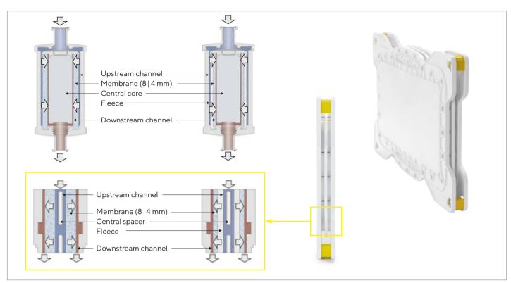
The direct comparison of capsule (upper cutaway) and cassette design (bottom) shows same construction principles, bed height and flow scheme.
