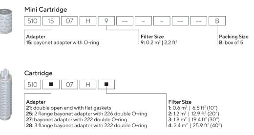
(Standard with silicone O-ring, optionally with EPDM O-ring. Example 5102507H1---E)
