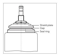
The cell has a rating of IP44 in normal weighing mode. This protection rating is only valid when there is a gap between the shield plate and the seal ring.
