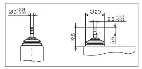
The transducer can be installed on this stud using clamps, for example. The transducer should consist of conductive, non-magnetic material in order to minimize electrostatic and magnetic interference. The transducer must weigh 5 g  $\pm$  0.1 g, so that the full weighing capacity of 20 g can be achieved. Additional preload must be smaller than 10 g in order to use the internal calibration function. Remove the transducer when transporting the weigh cell.
