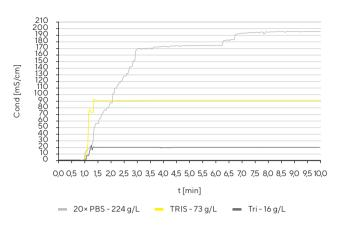
Fig. 1: General principle of mixing time determination via conductivity
