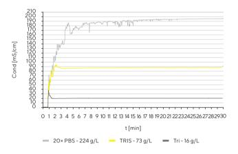
Fig. 4: Buffer preparations in 1000 L Flexel® Bag for Lev Mixer
