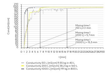
Fig. 5: PBS 20× buffer preparation in Flexel® Bag for Lev Mixer
