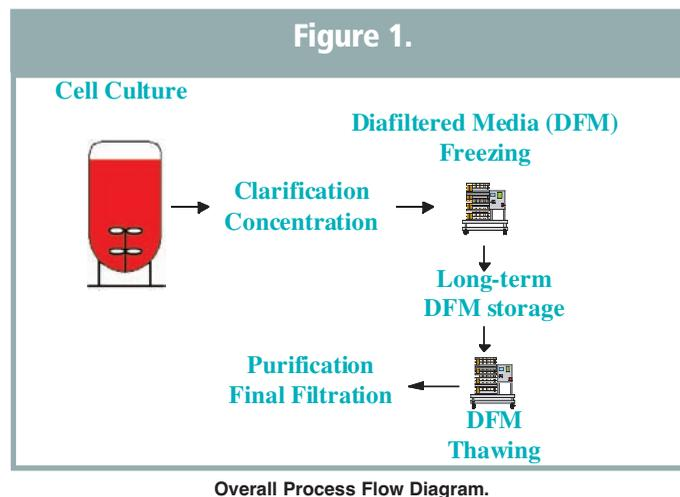
The long term storage allows for decoupling of the cell culture and harvest operations discussed above from the downstream purification process. The decoupling of the process provides operational flexibility for manufacturing between the cell culture and purification areas.
