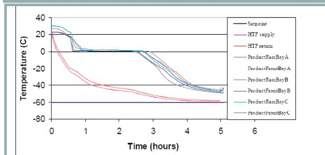
Freeze Profiles Shown to be Independent of Bag Placement. "HTF supply" and "HTF return" denotes the temperature of the heat transfer fluid when entering and exiting the freeze units. "ProductRearBayA" denotes the freeze profile for the bag placed in the front section of bay A. All other labels follow the same naming system.
