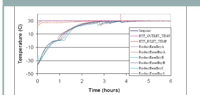
Thaw Profiles Shown to be Uniform and Reproducible. "HTF\_Outlet\_Temp" and "HTF\_Inlet\_Temp" denotes the temperature of the heat transfer fluid when entering and exiting the freeze units. "Setpoint" shows the target setpoint of the heat transfer fluid. "ProductRearBayA" denotes the freeze profile for the bag placed in the front section of bay A. All other labels follow the same naming system.
