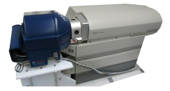
Note. An Applied Biosystems/ SCIEX 3200 QTRAP featuring hybrid triple quadrupole/linear ion trap capabilities was used for the mass spectrometry analysis. NanoESI was ensured by the TriVersa NanoMate, a chip-based ion source. The Agilent HPLC system is not shown. (Image credits: Department for Plant Biochemistry, Albrecht-von-Haller-Institute for Plant Sciences, Georg-August University of Goettingen, Germany.)
