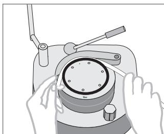
Thread the Sterisart® NF tubing in the pump head, following the instructions given for the pump used.
