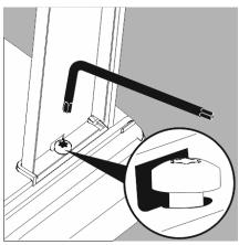
6) Turn the key approx. two times to loosen the Torx screws.
