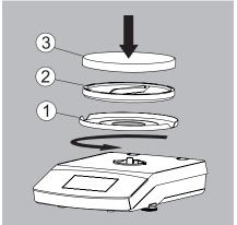
3) Install the pan support (1) and weighing pan (2).
