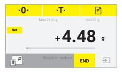
> The weighing display shows the step **Weight in medium**.
