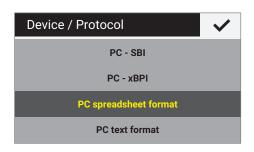
➤ To access the PC spreadsheet format menu option on the balance: Go to USB port and select the Device/Protocol option.
