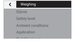
A number of basic settings for the weighing functions can be defined here. Options are limited for verified balances. All settings given in the menu are permitted.
