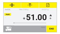
> The maximum measured weight value is displayed and kept as long as the sample remains on the balance.
