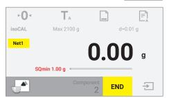
ightharpoonup The component is saved, and the balance is automatically tared.
