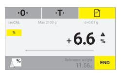
ightharpoonup The balance shows the percentage of the sample based on the reference sample.
