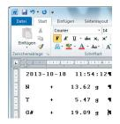
With the "PC text format" setting on the balance, Microsoft Word 2010 has the following display for the "Gross/Tare/Net" example:
