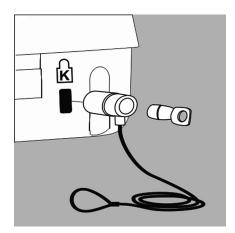
A "Kensington" key lock cable can be installed at the fastening point on the back of the balance if required.
